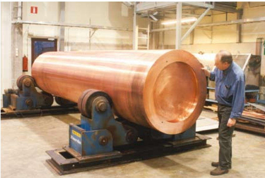
Copper cylinder for spent fuel disposal in Finland (courtesy Posiva)
