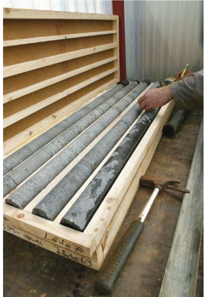
Measurements of drill cores from test drilling in Sweden (courtesy SKB)
