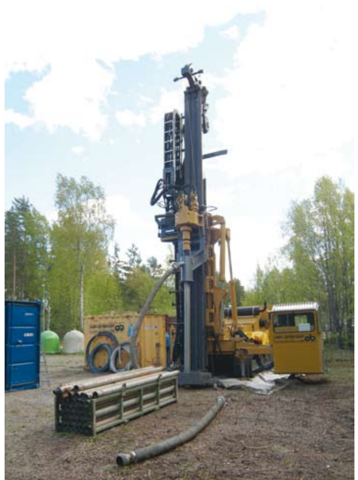
Borehole drilling during surface investigations in Sweden (courtesy SKB)
