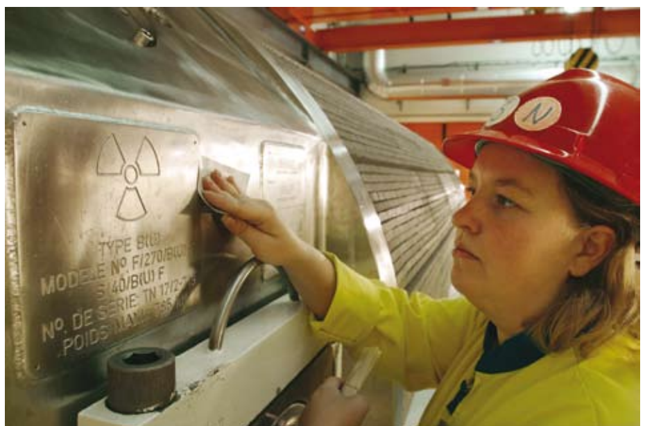
Transport cask in the reception area of the Swedish central interim storage facility for spent nuclear fuel (courtesy SKB)
